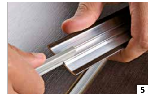
5) Keep the profile with the groove for insertion facing upwards and slot in the insert from the top downwards (if it does not slide easily, lubricate with water, silicone spray or vegetable oil).
